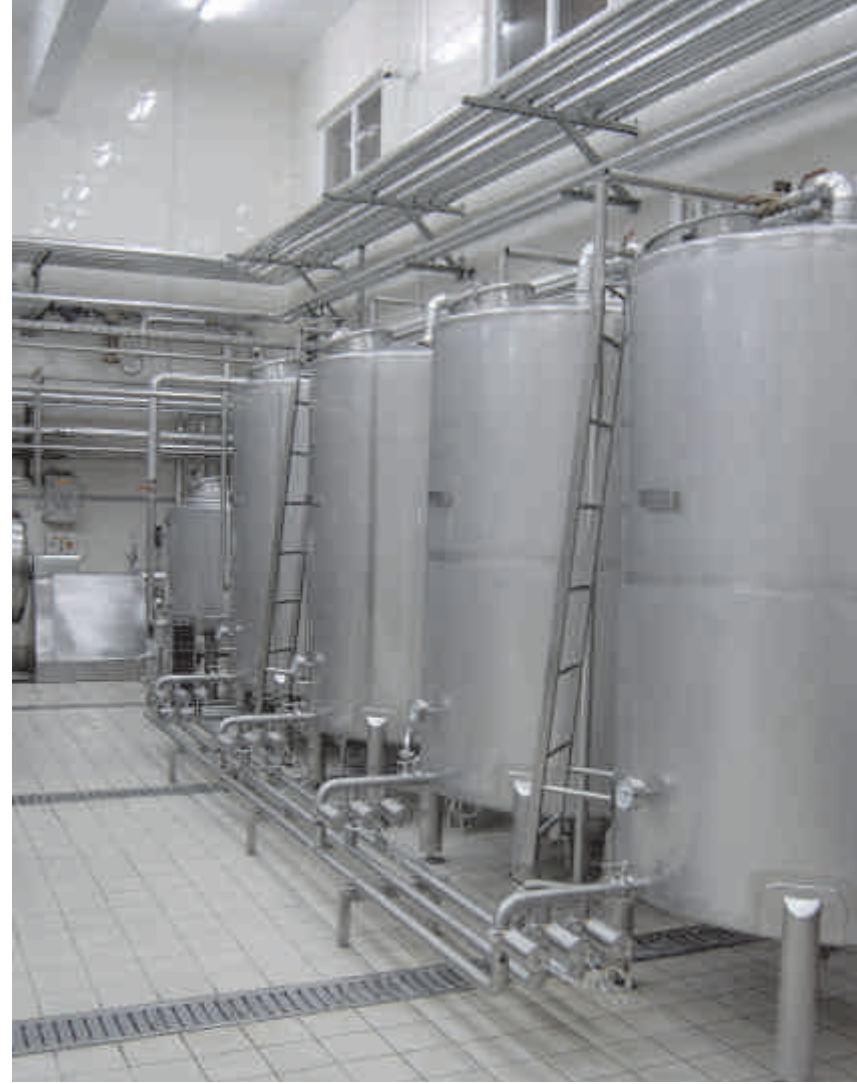
PLC Kontrollü CIP ÜNİTESİ CIP Unit with PLC Control
