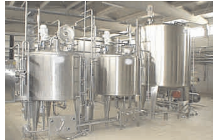
KREMA PROSES TANKLARI Cream Processing Tanks
