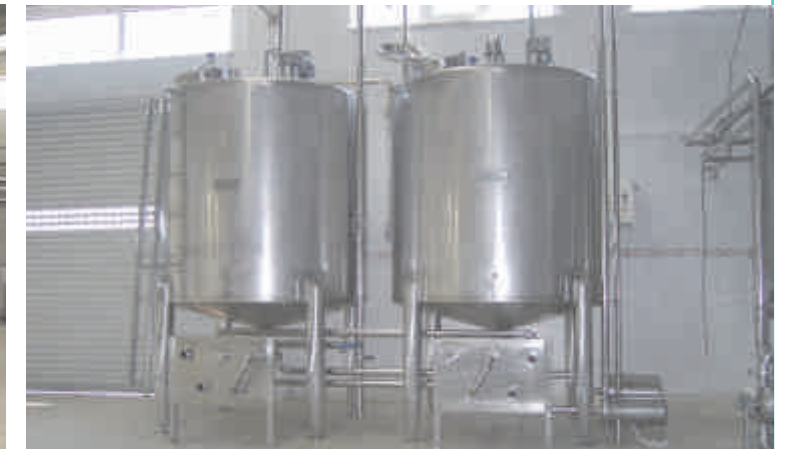
AYRAN PROSES TANKLARI Drinking Yoghurt Processing Tanks
